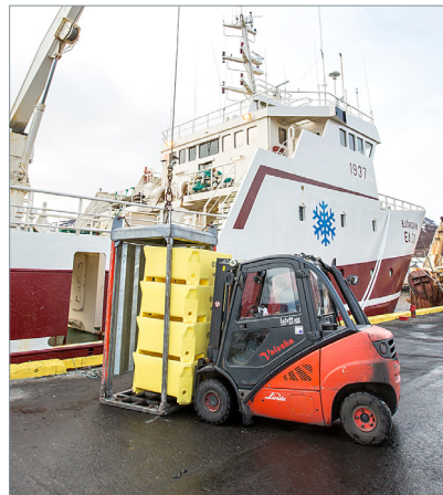
The cage opens and a fork lift can take out the stack.
